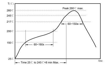
Preheat condition: 150 ~200 °C / 60~180 sec. Allowed time above 217 °C : 60~150 sec. Max temperature: 260 °C. Max time at max temperature: 10 sec.
