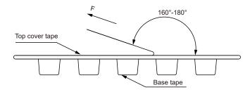
The peel force of top cover tape shall be between 0.2 to 1.17 N
