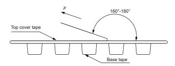
The peel force of top cover tape shall be between 0.1 to 1.17  $\mbox{N}$
