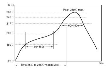
Preheat condition:  $150 \sim 200 \degree / 60 \sim 180$  sec. Allowed time above  $217 \degree : 60 \sim 150$  sec.
