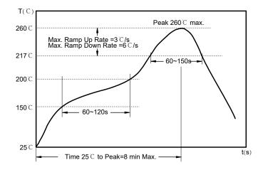
Preheat condition:  $150 \sim 200 \text{ C} / 60 \sim 120 \text{ sec.}$ Allowed time above  $217 \text{ C} : 60 \sim 150 \text{ sec.}$ Max temperature: 260 C. Allowed Reflow time: 2x max.
