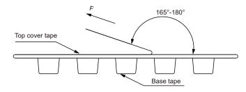
The peel force of top cover tape shall be between 0.1 to 1.3 N
