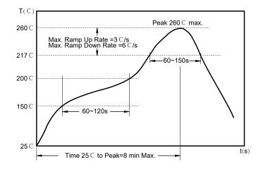
Preheat condition:  $150 \sim 200^{\circ}$ C /  $60 \sim 120$  sec. Allowed time above  $217^{\circ}$ C :  $60 \sim 150$  sec. Max temperature:  $260^{\circ}$ C. Allowed Reflow time: 2x max.
