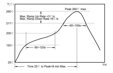
Preheat condition:  $150 \sim 200$  °C /  $60 \sim 120$  sec. Allowed time above 217 °C :  $60 \sim 150$  sec. Max temperature: 260 °C . Allowed Reflow time: 2x max.
