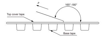
The peel force of top cover tape shall be between 0.1 to 1.3 N
