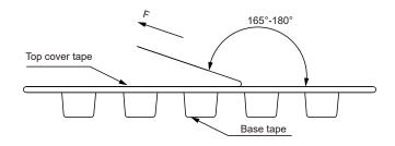
The peel force of top cover tape shall be between 0.15 to 0.78 N
