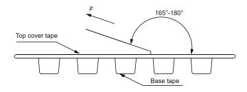
The peel force of top cover tape shall be between 0.14 to 0.78 N
